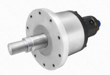
Specialized Example 2 - designed for an uncoiler / recoiler expanding mandrel application. Design features a complete assembly solution integrating a rotary union, rotating cylinder (for actuating the expanding mandrel), and position sensor.
